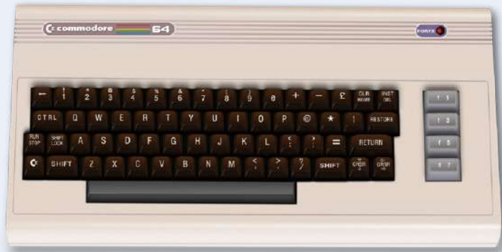
Figure 3: The Commodore 64, one of the famous home computers from the 1980s, has a 6502 inside. (Source: ralfsfotoseite @ Pixabay)
