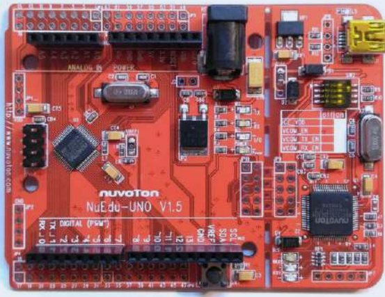
Figure 5: The Nuvoton NuMaker Uno board has a detachable NuLink programmer/debug module. (Source: https://danchouzhou.blogspot.com )
