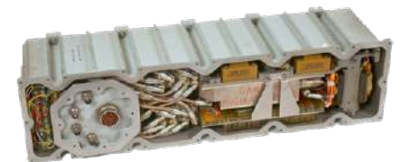
Figure 3: Operating at several thousand volts, the Collins Radio amplifier was a tightly-packed tangle of coaxial cables. (Source: Ken Shirriff)
