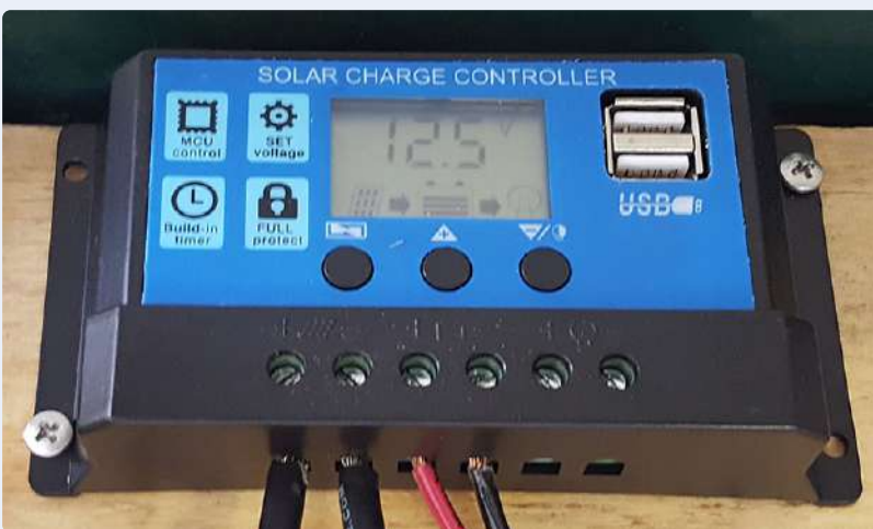
Figure 5: Charge controllers that look like this one certainly do not have MPPT functionality (even if they carry a sticker bearing those letters!). (Source: United States Department of Energy)
