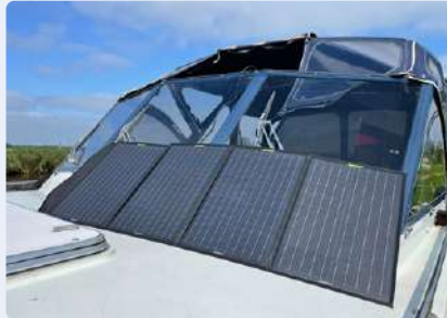
Figure 9: The foldable solar panel chosen by both Martin and Detlev can be stored below deck when underway. It is rated at 120 Wp. (Source: Martin Jepkens)
