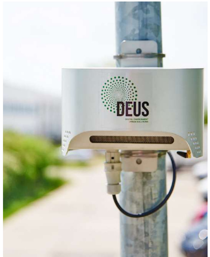
Figure 5: DEUS POLLUTRACK particulate matter sensors gather data from stationary and mobile IoT units. Data is delivered to the back-end using 4G and 5G cellular networks. (Source: DEUS POLLUTRACK)
