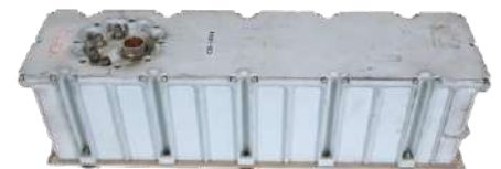
Figure 2: Collins Radio S-Band traveling-wave tube amplifier used for communication with earth during the Apollo mission. (Source: Ken Shirriff)
