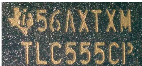
▶ Figure 5: The logo on this TL082 looks a lot like, but is not identical to, a real Texas Instruments logo on a 555.
