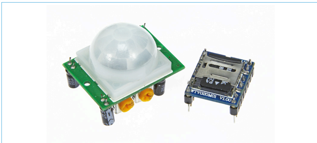
Figure 2. The sound module and IR sensor module used in the project.
