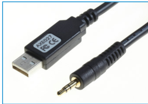
Figure 2. USB-to-serial cable. Looks familiar, doesn't it?
