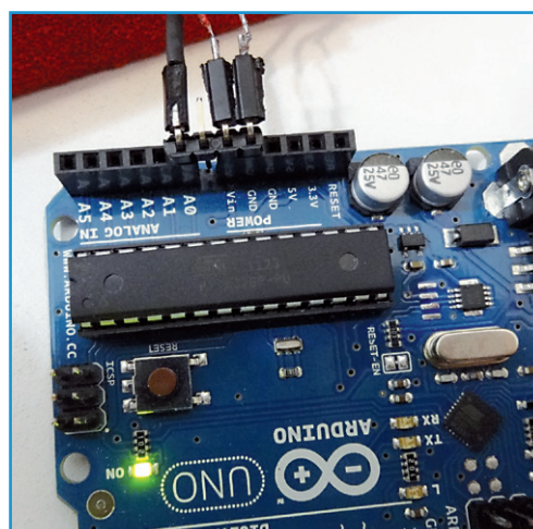
Figure 1. Connecting the probe to your UNO board.
