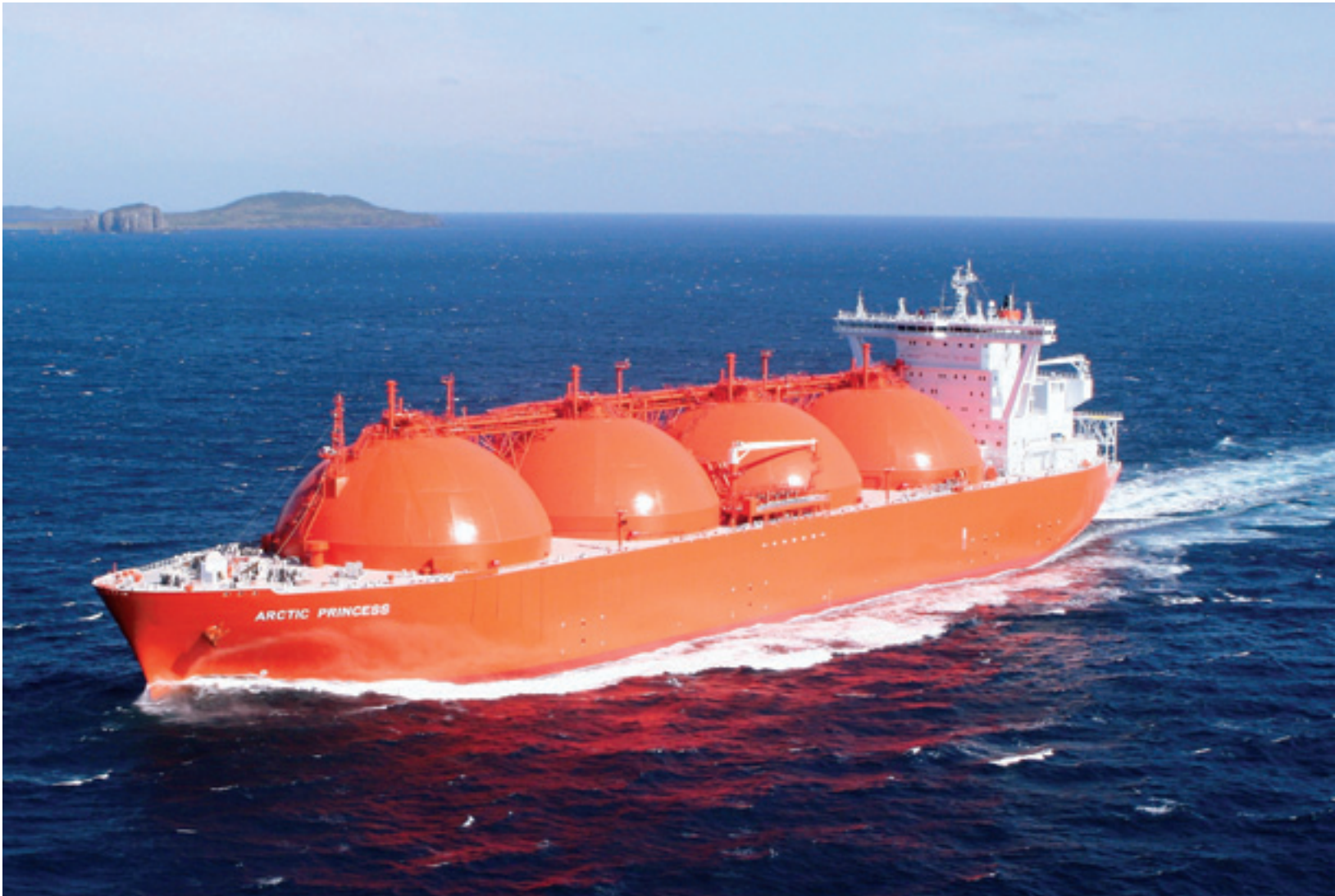
The Arctic Princess has a capacity of 147,000 cubic metres of LNG, sufficient to cover the yearly energy consumption of all households in a city with a population of 45,000 people.
