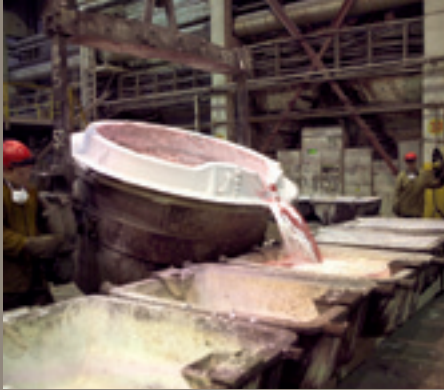
Melted aluminum is poured in moulds at Rusal's Bratsk aluminum smelter. Photo: Rusal
