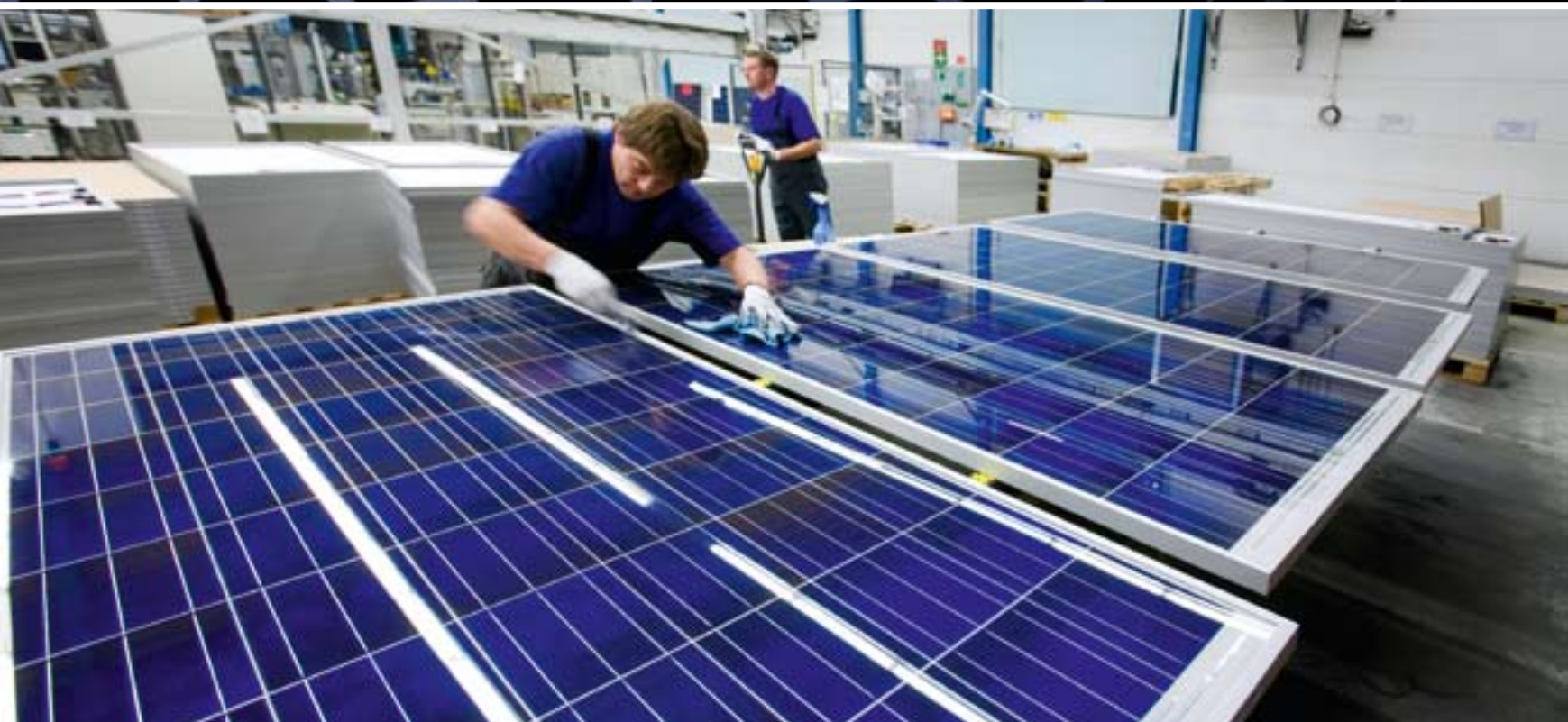
Manufacturing of solar power panels at Deutsche Solar. Photo: Rainer Weisflog
