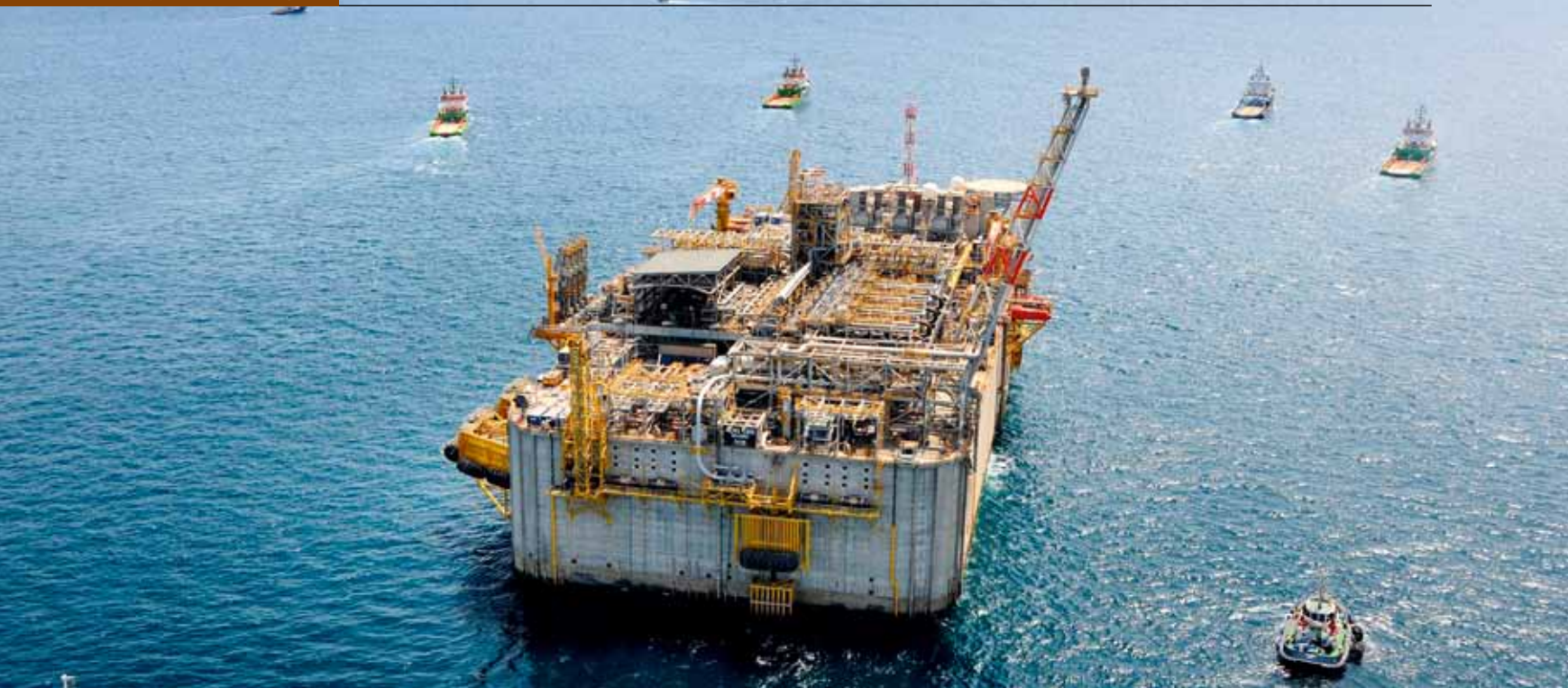
The Adriatic LNG terminal being towed from Algeciras (Spain) to Italy. Photo: EPA/Business Wire
