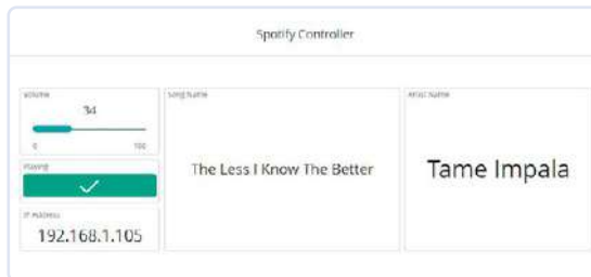
Figure 12: Current song and artist name are sent to the Arduino Cloud, where they are visible on your personal dashboard.
