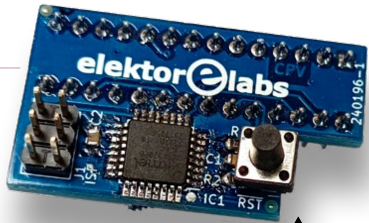
Figure 4. The ATmega328PB-to-STC15W408AS adapter board, configured for software development.
