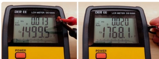
Figure 4: These reference capacitors of 1 nF each are not the best.
