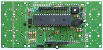
Platino likes to be the centre of attention. He therefore has invested in a buzzer to ensure no one ignores him. To prevent him becoming hoarse he always uses the buzzer with a current-limiting series resistor (R2).
