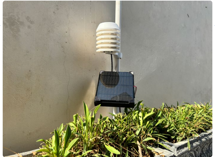
Figure 18: LoRa Sensor Node deployed.
