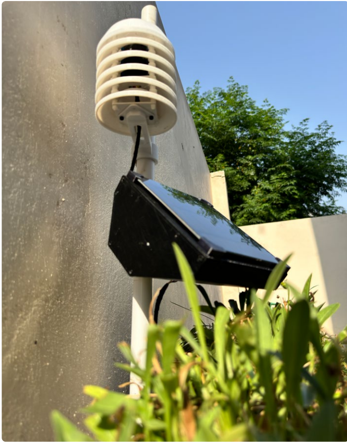
Figure 17: Low-angle view of the LoRa Sensor Node, showcasing the Stevenson enclosure.
