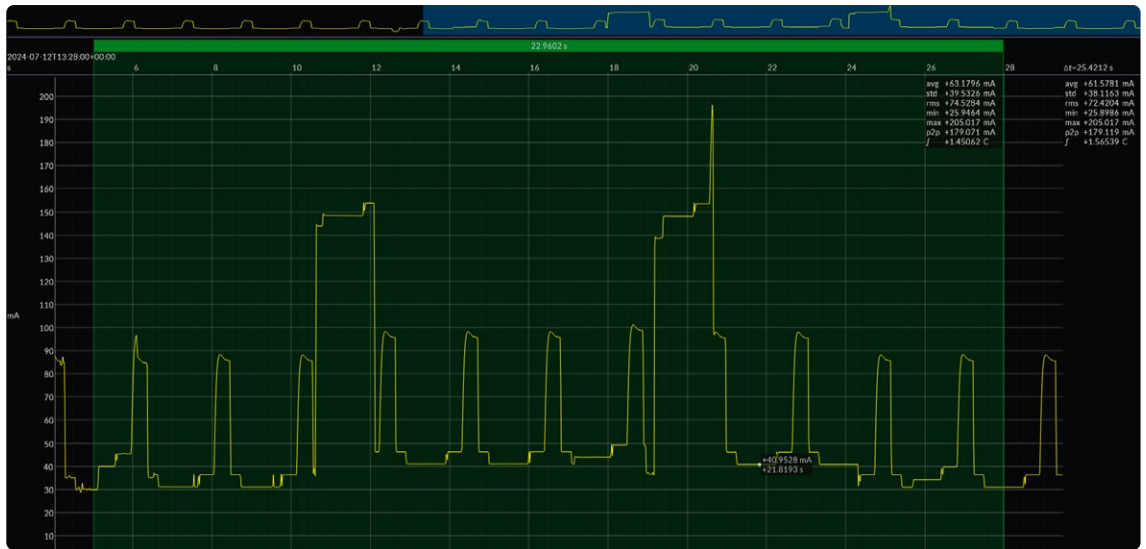
Figure 10: The current waveform of the SCD30 and LoRa Module.
