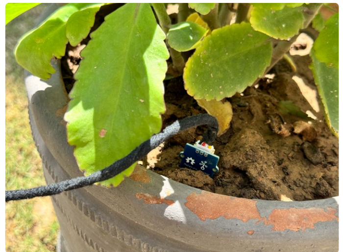
Figure 3: The soil sensor. As it has open pads and the JST connector, it can cause a short circuit if it catches moisture.
