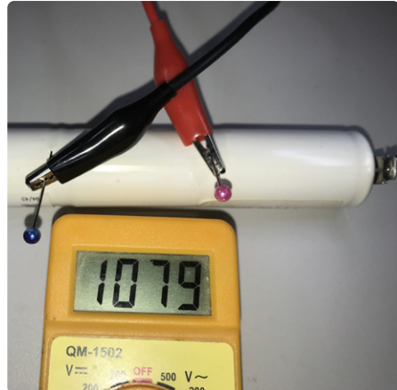
Figure 3: Using dressmaking pins to measure the voltage of a (rather flat) Ni-Cd cell in a pack.
