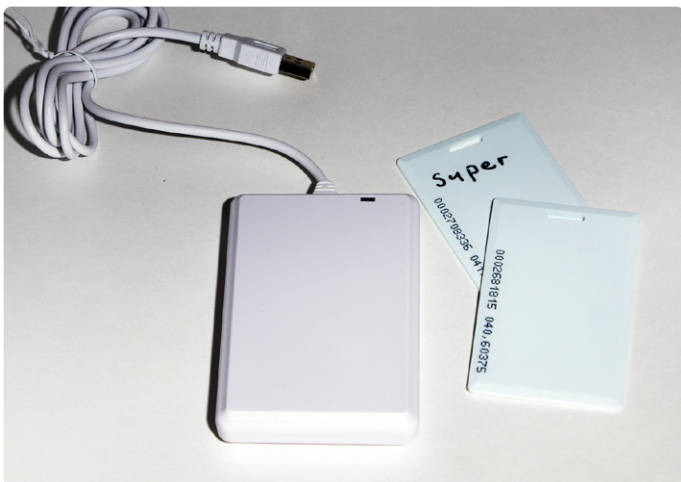
Figure 12: A USB-controlled RFID card reader suggested as part of the human interface section.
