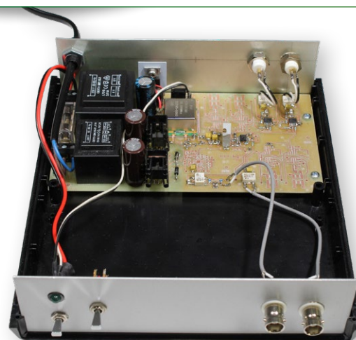
Figure 4: A partially assembled circuit board installed in a Teko housing.
