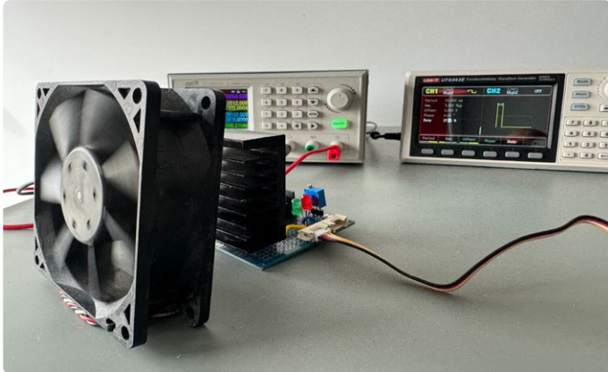
Figure 2: Test setup, with using a function generator to control the circuit via PWM.
