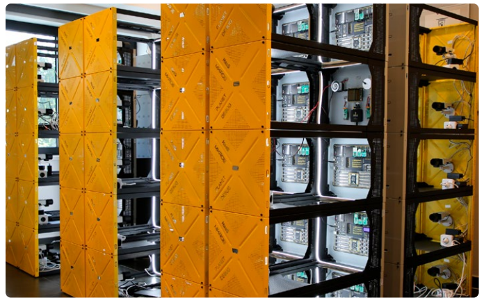
Figure 1: Planet Debug's remote stations with 130+ development boards, including MCU cards, peripherals, and displays — no need for costly hardware.
