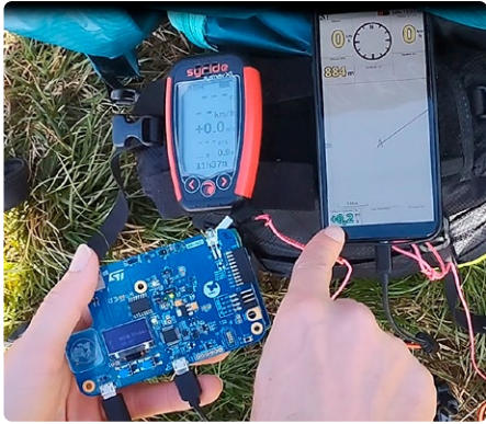
Figure 5: A commercial variometer was used to compare measurements made with my Open Vario.
